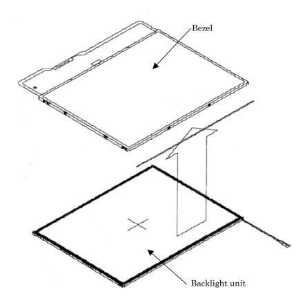
Figure 4-53 Replacing TMD fluorescent lamp (WXGA) (3)
